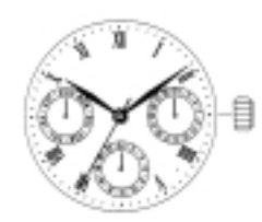
6P29 height 3.45mm 3 eyes (Day/Date/24 hour) 3 year battery life (SR621SW)
