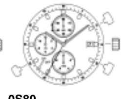
OS80 height 4.68mm date chrono hour/min/sec +1/20 second alarm 2 year battery life (SR927W)
